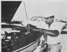
Silvio Cijntje di E. R. Safety inspects the battery cable to prevent a short circuit, which could cause a fire.
